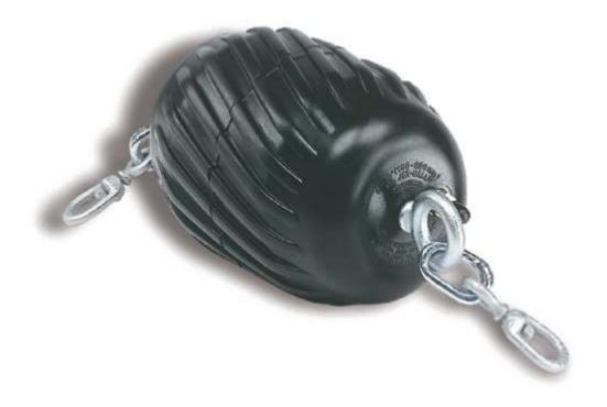
The 109 Series pipeline cleaning ball uses the force of water to spin and scrub pipes clean. The ball's spiral ribs create the spin, while eyebolts on each end of the ball allow it to move in either direction through pipe. The following instructions describe how to install and operate your cleaning ball.
