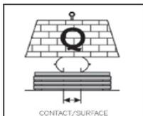
With the Lift Bag fully inflated, the contact surface and lifting capacity reach their minimum, and the lifting height its maximum (**Figure 3**). To be able to correctly operate the Lift Bag, a user must understand the data relating to the maximal lifting force, maximal lifting height, and maximal lifting capacity at maximal lifting height.
