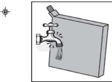
Rinse the surface with cold, fresh water (**Figure 14**) or with a water jet to remove all remaining dirt and detergent. With the air bag in the upright position, wipe the nozzle with clean dry cloth. Let the air bag dry in an open dry atmosphere. Don't speed up drying with heat.
