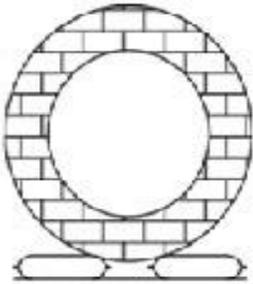
Cylindrical objects of great size such as tanks don't admit lifting by a single Lift Bag. If the object is not firmly fastened it will roll away when the Lift Bag begins inflating to its typical spherical form. Cylindrical objects must be lifted using two Lift Bags, one at each side of the object. The inflation must be controlled to permit equal coordinated lifting (**Figure 11**).
