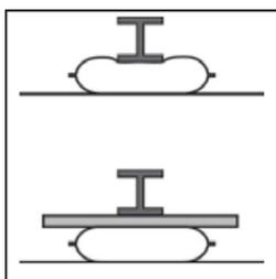
The Lift Bag steel or Kevlar cord can be damaged by twisting if the load does not contact the entire surface of the Lift Bag. A support must be inserted between the Lift Bag and the load to permit the lifting force to be equally distributed over the entire lifting surface (**Figure 10**).
