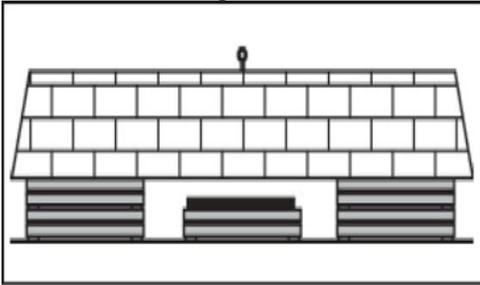
mm (2.76") space between the ground and the object to be lifted, build a firm foundation leaving just enough space to insert a non inflated bag onto the foundation and under the load. The foundation must be undivided without any gap under the Lift Bag (**Figure 5**). Add safety supports to each side of the Lift Bag/s as the load is lifted (**Figure 5**) to support it in the event the Lift Bag or inflation system fails.
