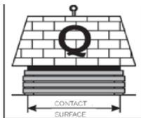
Position the Lift Bag on a level foundation (**Figure 1**). The fully deflated Lift Bag contains very little air.
