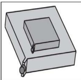
In order to increase lifting height it is also possible to use two air bags. Place the smaller one in the middle and on top of the larger one, with the inflation nozzles pointed away from the load (**Figure 7**). Never stack more than two air bags under a load.
