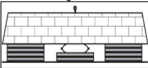
After each time the load is lifted, slowly empty the Lift Bag lowering the load onto the safety supports.
