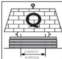
During the process of Lift Bag inflation, the air column and consequently the lifting height are increasing, while the contact surface between the bag and the object is decreasing, resulting in decreasing lifting capacity (**Figure 2**). Thus, maximal force can be attained only at the beginning of inflation, when the lifting height is minimal. During the inflation, the air bag is gradually getting a characteristic spherical form.
