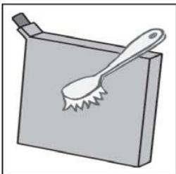
Clean the Lift Bag surface with a brush with hard bristles moving the brush in all directions. Never use a sharp brush that might damage the Lift Bag. After brushing off the dirt, use a brush to wash off any remaining oil or dirt with a light solution of warm water and a dish washing detergent using the brush (**Figure 13**).
