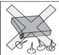
Position the Lift Bag on a flat surface cleared of any glass fragments or other foreign particles that might damage it. Use sand or another granulated material to cover any slippery surface such as oily spots or ice - to reduce the risk of slipping. When the Lift Bag area is soft, unstable not level, build a solid support (**Figure 4**).
