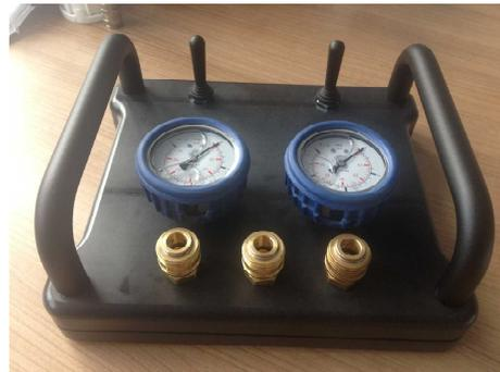
This has two separate lines allowing for the independent inflation of 2 lift bags.
