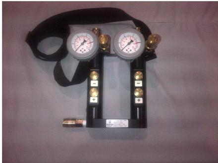
This has one or two separate lines allowing for the independent inflation of 1 or 2 lift bags.
