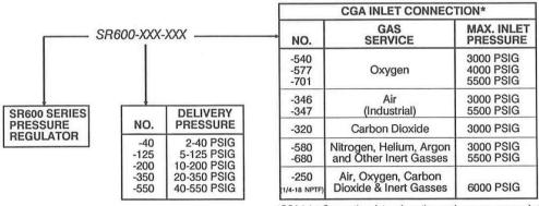
\*CGA Inlet Connection determines the maximum recommended inlet pressure
