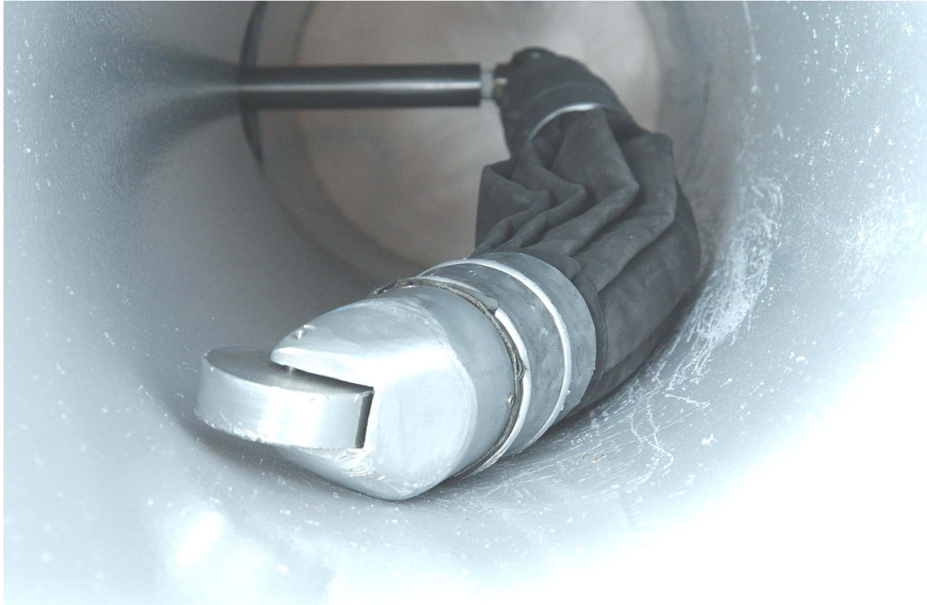
The MultiFlex Plug shown entering tapped pipeline
