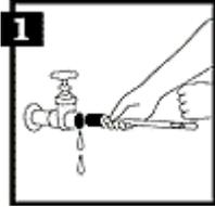
Shut off main water source and insert the Plug through the open valve that is to be repaired.
